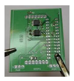
• Thru-hole components: components with leads that go through the circuit board and get soldered on the other side.
